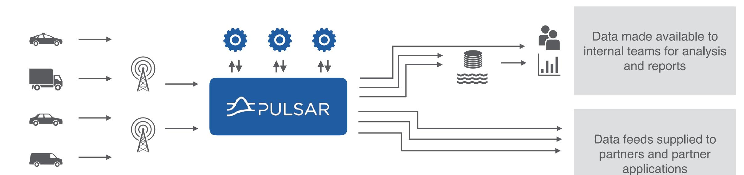
Telemetry data from connected vehicles transmitted and published to Pulsar
